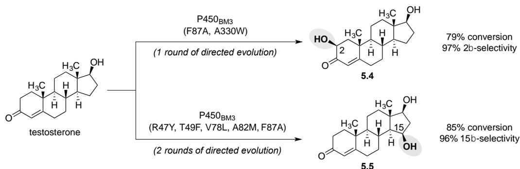
**Figure 5.5.** Regiodivergent hydroxylation of testosterone by engineered P450<sub>BM3</sub> variants (21).
